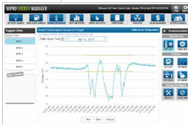
Figure 3: Snapshot of Wipro Energy Manager Application showing a Teller Area's Temperature trend at a site
